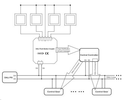
The SYMPHO DALI2 Push-Button Coupler supports 4 instances (1 - 4) of type 1 (IEC62386-301, Input Devices - Push Button) which are assigned to the 4 button inputs.
