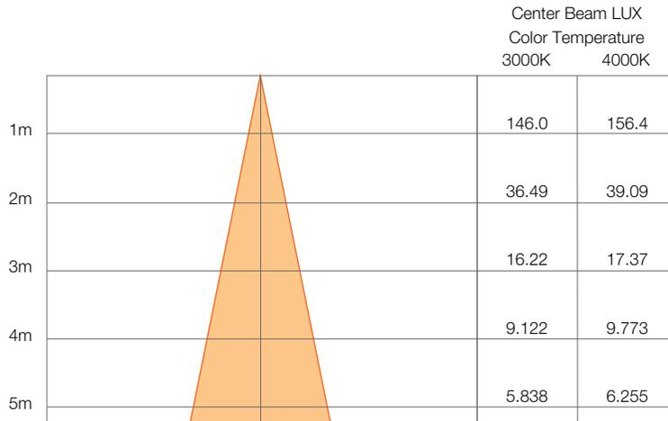
Diagram based on Diffused Prism 3000K measurement
