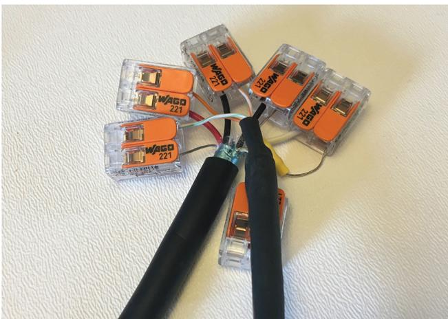
Figure 23 – DMX Termination Detail
