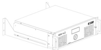
Make sure that the server rack is sufficiently ventilated and proper cage nuts and rack screws are used.
