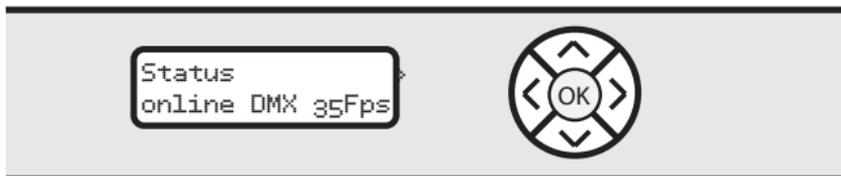
After powering up the Butler PRO DC, the loader shows the loading progress and revision levels of the loader and the firmware. After loading is completed, the Butler PRO DC enters operational mode. The setup mode must be selected separately.
