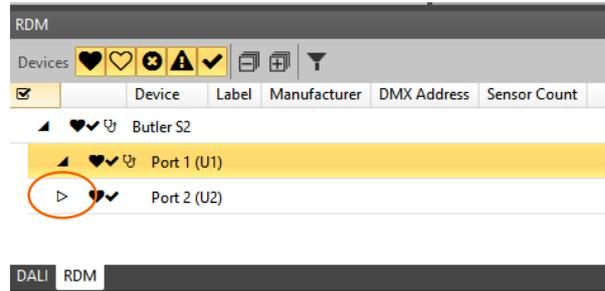
7. Click the triangle arrow and the list will expand revealing all of the detected devices on the output port of the output device.
