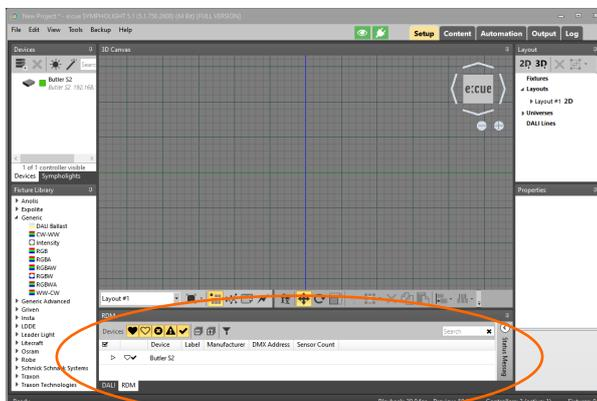
4. Enable RDM mode for the output device by right clicking on the output device and select **Enable RDM**.
