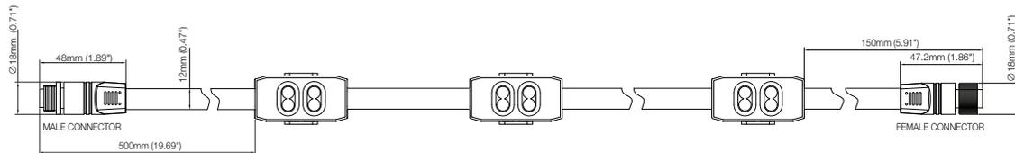
NOTE: Cable and connector dimensions are the same for ARCHISHAPE® 2.0 Dot M and L.
